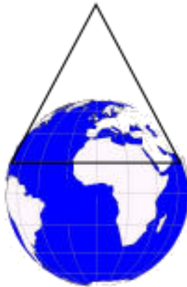
Figure: Globe with Conic Projection
